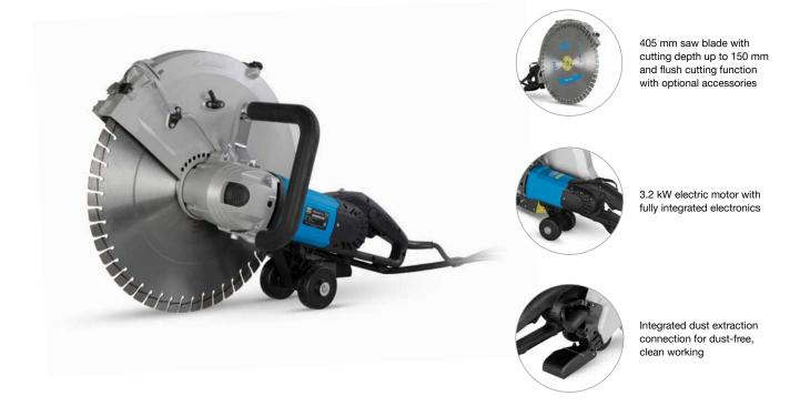
The HBE400\*\*\* is a 3.2 kW handheld saw for cutting depths up to 150 mm. In combination with our accessories kit, this hand-held saw is excellently suited to flush cutting. This model can be used for both wet and dry applications and its integrated dust extraction connection enables clean working. The compact design, low weight and detachable guide rollers guarantee ease of handling and machine guidance for the user. The 230 V electric drive enables flexible working indoors and outdoors.
